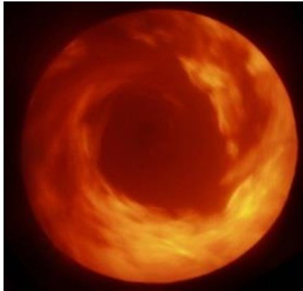
View into the vortex of ABC's TORBED EBR as it combusts rice husks
